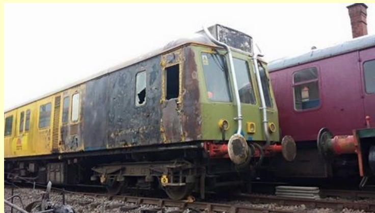
Class 121 55029 damaged by fire, 25/5/15 (D.West)
